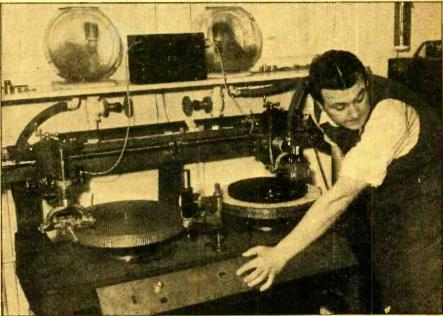
At Sosnik's signal, recorder Donald Thompson adjusts wax and needle in the control-room and two "takes" are made. Thompson scrutinizes the revolving wax through a microscope to be sure the needle is cutting the proper depth
